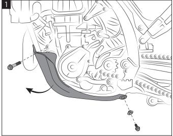
If present, remove the original skid plate by unscrewing the screws and the bushing as shown in the figure. Otherwise, just remove the screws in the frame.
