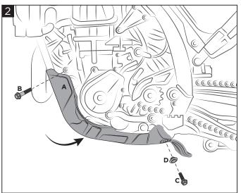
Position the Acerbis skid plate (A) and fix it using the supplied screws (B), the bushings (D) and the second screws (C).
